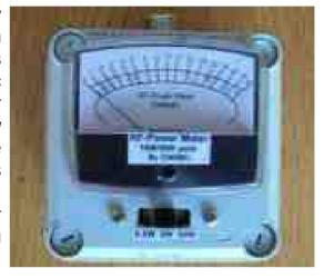
This RF-power meter combined with build-in dummy load is made to measure power levels starting from a few milliwatt up to 50 watts (or more if suitable components are used and more then diode is used). IT has 3 scale readings: 0.5 watt, 5 watt and 50 watts. Again, you can extend the scales easily. The power meter is ideal for measuring QRP levels.
