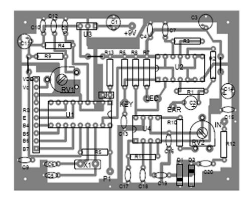
The whole circuit is mounted on a 60x80 mm PCB board. It is recommended to make use of small sized components (ceramic multilayers capacitors, low voltage electrolitics, ...) so as to make easier the assembling. The LCD display is connected by a 10 pole flat cable soldered to 2.54 mm standard connectors, as shown below
