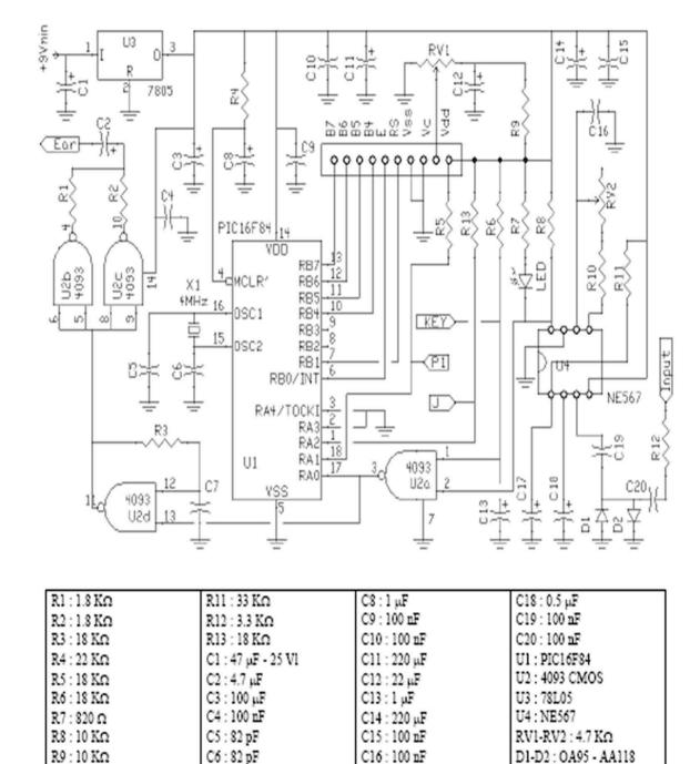
The schematic appears very simple, actually almost all of the functions are performed by the microprocessor software, while an NE567 tone decoder takes charge of processing the audio input signal. This IC contains a PLL circuit whose lock frequency may be adjusted between 700 and 1000 Hz by the RV2 trimmer.
