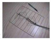
the size of the antenna. I was always satisfied with the antenna and a direct comparison to other antennas of a know gain showed that it really has to a have a gain of about 10dB over a dipole.
