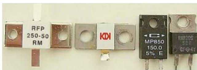
Being a passive-grid amplifier, most of the input power is dissipated in a non-inductive  $50\ \Omega$  resistor, see four types, left to right:
