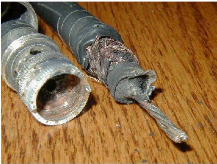
This is what happens to a PL-259 with 1500 watts applied and the antenna is NOT resonant. This was on my double bazookas and I was attempting to load them up on 20 meters with a tuner. *Sparks, Flames and Pouf*
